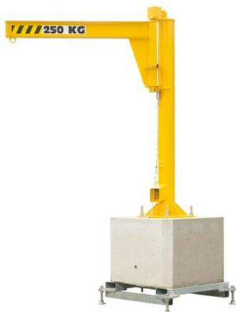
The headroom is the main asset of the PFI MOB. Appropriate for an indoor or outdoor use, its I beam profile allows to consider installation of a hoist with electric or manual steering. This jib crane is mounted on a movable concrete block provided. Displacement can be done by traveling crane (transport ring) or by forklift.
