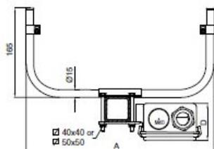
A towing arm is attached to the moving machinery and connected to the collector trolley via chains. The arrangement is such that when pulling in either direction one of the collector towing chains is taut, the other remaining slack. In this way lateral movements of the crane, hoist, etc. are not transmitted to the trolley. This tolerance provides ultimate security of service!
