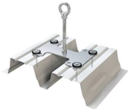
Stainless steel anchor point ABS-Lock X-T-21 (Ø 16 mm) and base plate (290 x 200mm) is a fall protection solution developed for usage on a warm roof. The anchor point is easily installed using the 4 specially prepared toggle bolts included in the package. Distance between the pred-drilled holes: 180 - 250 mm
