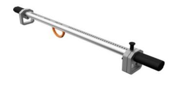
JAMBTAC Mobile Door Truss. Mobile anchoring point for all door widths from 600 to 1,100 mm. The adjustable mobile door truss made of aluminium is very light and can be easily adapted to different door widths. Rounded profile edges and plastic caps at the ends reduce the wear of material, the risk of injuries for the user and prevent the door posts from being scratched. JAMBTAC can be used simultaneously by up to two persons.
